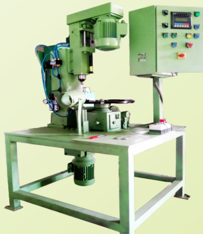
Drilling & Chamfering SPM with Cam Index, PLC & Auto Unloading
