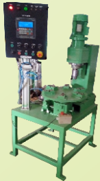
SPM with Spin Riveting, Fixtures Cam Index, PLC & Auto Unloading
