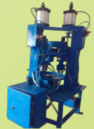
Dual Drilling & Tapping SPM, Cam Index, PLC & Auto Unloading
