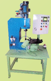
SPM with Hydro Pumatic Press, Cam Index, PLC & Auto Unloading
