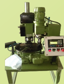
Drilling & Tapping SPM, Cam Index, PLC & Auto Unloading
